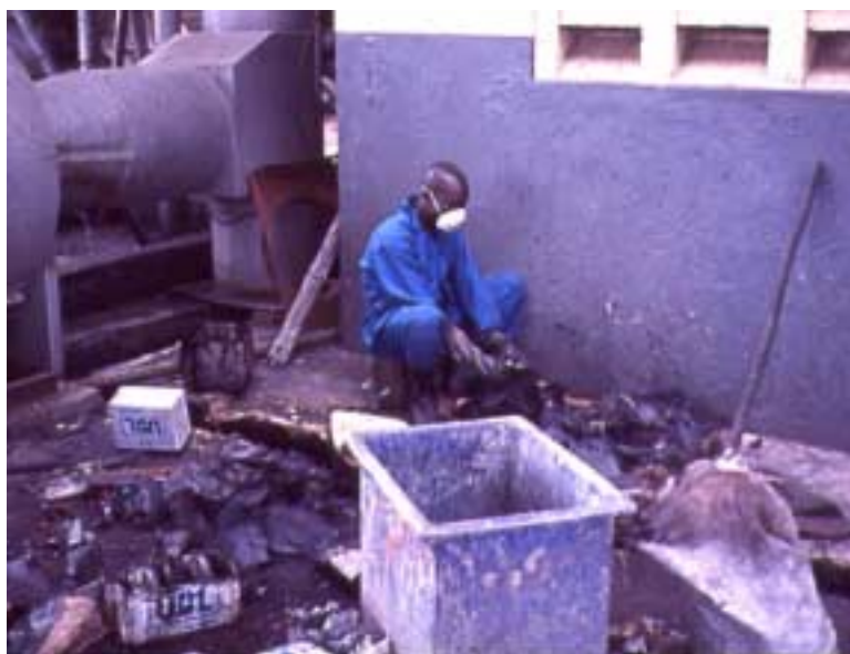
Figure 10: Recycling at UBL. Batteries are dismantled as showed in the picture, then the lead plates are melted, and formed into new plates. (Photo from field study)
